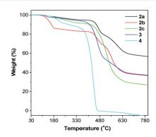
Fig. 1 TGA curves of TPE-Pys recorded under nitrogen at a heating rate of 10 °C min<sup>-1</sup>
