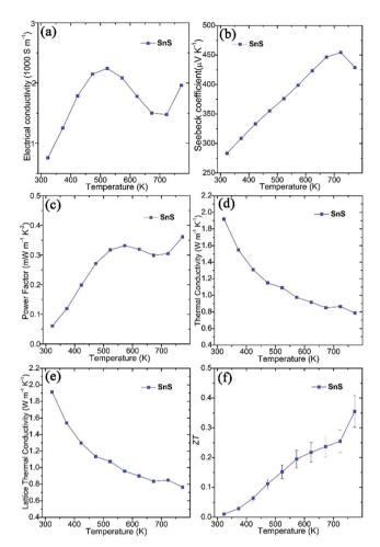
Fig. 2 Thermoelectric properties of SnS pellets sintered using SPS, measured perpendicular to the pressing direction: (a) the electrical conductivity  $(\sigma)$ , (b) the Seebeck coefficient (S), (c) the power factor  $(S^2\sigma)$ , (d) the thermal conductivity  $(\kappa)$ , (e) the lattice  $\kappa$   $(\kappa_L)$ , and (f) ZT as a function of temperature.
