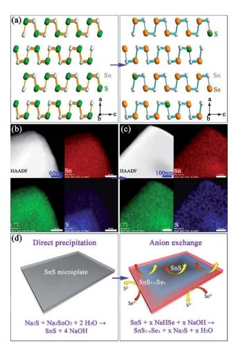
Fig. 3 Structure, composition and formation mechanism of Sn(S,Se): (a) structural models of SnS and SnS<sub>0.1</sub>Se<sub>0.9</sub>; elemental mapping of isolated plates after anion exchange for (b) 1 min and (c) 2 h; (d) schematics of the initial precipitation and subsequent exchange processes. The four panels in (b) and (c) show the high angle annular dark field (HAADF) image of a plate and corresponding elemental maps for Sn (red), Se (green) and S (blue) respectively.
