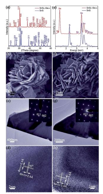
Fig. 1 Characterisation of SnS (a–e) and  $SnS_{0.1}Se_{0.9}$  (a, e–h) nano/micro-plates: (a) PXD data; (b, f) SEM images; (c, g) TEM images of individual plates and corresponding SAED patterns along the [100] zone axis (inset); (d, h) HRTEM images of plates with d-spacings indicated, (e) EDS spectra collected from isolated plates.
