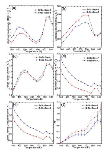
Fig. 5 Thermoelectric properties of SnS<sub>0.1</sub>Se<sub>0.9</sub> pellets SnS<sub>0.1</sub>Se<sub>0.9</sub>-1 and SnS<sub>0.1</sub>Se<sub>0.9</sub>-2 measured perpendicular to the pressing direction: (a) the electrical conductivity  $(\sigma)$ , (b) the Seebeck coefficient (S), (c) the power factor  $(S^2\sigma)$ , (d) the thermal conductivity  $(\kappa)$ , (e) the lattice  $\kappa$   $(\kappa_1)$ , and (f) ZT as a function of temperature.
