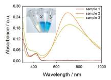
Fig. 3 UV-vis spectra and digital image (inset) of several reaction systems: FeCl<sub>3</sub>/K<sub>3</sub>Fe(CN)<sub>6</sub> (1), FeCl<sub>2</sub>/K<sub>3</sub>Fe(CN)<sub>6</sub> (2), and FeCl<sub>3</sub>/  $K_3Fe(CN)_6/H_2O_2$  (3). Reaction conditions: 0.25 mM FeCl<sub>2</sub>, 0.25 mM FeCl<sub>3</sub>, 0.25 mM  $K_3$ Fe(CN)<sub>6</sub> and 1 mM  $H_2$ O<sub>2</sub> in 50 mM MES (pH 3.0) at 25 °C, reaction for 10 min.
