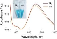
Fig. 4 UV-vis spectra of FeCl<sub>3</sub>/K<sub>3</sub>Fe(CN)<sub>6</sub>/GOx/glucose under air and nitrogen. Reaction conditions: 0.25 mM FeCl<sub>3</sub>, 0.25 mM K<sub>3</sub>Fe(CN)<sub>6</sub>,  $0.05 \,\mathrm{mg}\,\mathrm{mL}^{-1}\,\mathrm{GOx}$ , and 1 mM glucose in 50 mM MES (pH 3.0) at 25 °C, reaction for 10 min.
