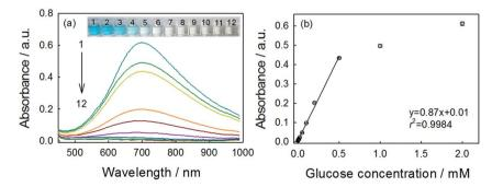
Fig. 5 UV-vis spectra (a) of different concentrations of glucose in the presence of 0.05 mg mL $^{-1}$  GOx, 0.75 mM FeCl<sub>3</sub> and 0.75 mM K<sub>3</sub>Fe(CN)<sub>6</sub> in 50 mM MES (pH 3.0) reaction for 10 min. Glucose concentrations (all in mM) from top to bottom (1 to 12): 2, 1, 0.5, 0.2, 0.1, 0.05, 0.02, 0.01, 0.008, 0.004, 0.001, and 0. The inset represented the corresponding samples. The linear relationship between the absorbance and concentrations of glucose (b) was also given.
