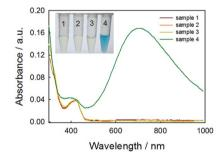
Fig. 1 UV-vis spectra and digital image (inset) of several reaction systems: FeCl<sub>3</sub>/K<sub>3</sub>Fe(CN)<sub>6</sub> (1), FeCl<sub>3</sub>/K<sub>3</sub>Fe(CN)<sub>6</sub>/qlucose (2), FeCl<sub>3</sub>/  $K_3Fe(CN)_6/GOx$  (3), and  $FeCl_3/K_3Fe(CN)_6/GOx/glucose$  (4). Reaction conditions: 0.25 mM FeCl<sub>3</sub>, 0.25 mM  $K_3$ Fe(CN)<sub>6</sub>, 0.05 mg mL<sup>-1</sup> GOx, and 1 mM glucose in 50 mM MES (pH 3.0) at 25 °C, reaction for 10 min.
