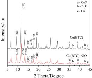
Fig. 3 XRD patterns of Cu(BTC) and Cu(BTC)-rGO.
