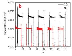
Electric current densities with different cathodes used: Cu(BTC)-rGO/Pt-Cu foam cathode (a), Cu(BTC)/Pt-Cu foam cathode (b).
