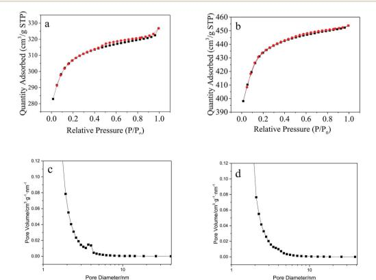
Nitrogen sorption isotherms: Cu(BTC)-rGO (a), Cu(BTC) (b); pore size distribution: Cu(BTC)-rGO (c), Cu(BTC) (d).
