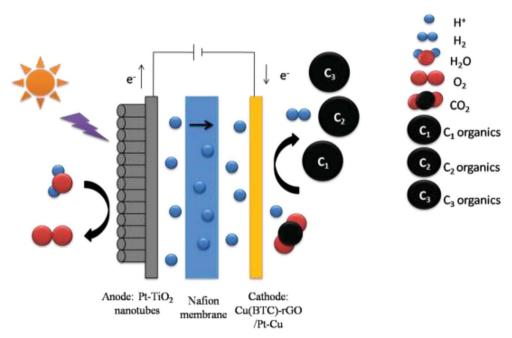
Fig. 1 Schematic of photoelectrochemical cell for CO<sub>2</sub> reduction.
