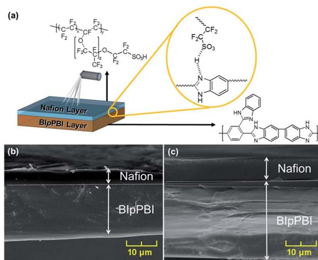
Fig. 1 (a) Schematic of the BI<sub>p</sub>PBI/Nafion hybrid membrane and its interface; cross sectional SEM image of (b) B20N5 and (c) B20N10.
