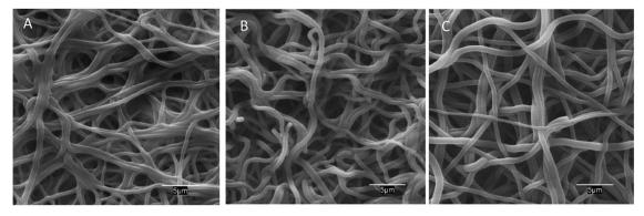
Fig. 2 SEM images of PAA-PVA fibres before impregnation (A), and dressings after impregnation (pH 7) nisin (N\_2@PAA-PVA, (B)) and lysozyme (L\_2@PAA-PVA, (C)).
