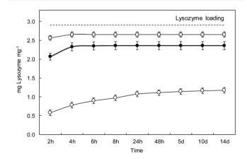
Fig. 7 Release of lysozyme in different media: phosphate buffer saline pH 7.4 ( $\odot$ ), carbonate buffer pH 10.0 ( $\square$ ) and acetate buffer pH 3.5 ( $\bigcirc$ ). The dashed line represents the lysozyme loading of specimens L\_1@PAA-PVA.
