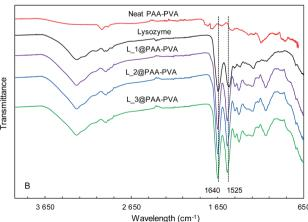
Fig. 1 FTIR-ATR spectra of PAA-PVA functionalized dressings. Nisin (A) and lysozyme (B) functionalized at pH 7 (the spectra for dressings functionalized at pH 10, are shown in Fig. S1†).
