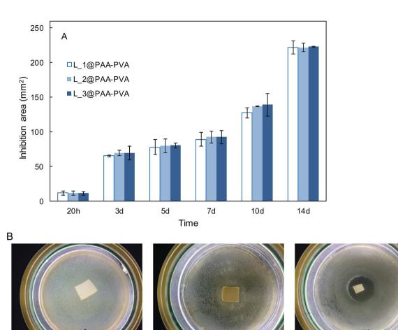
Fig. 4 Halo inhibition zone expressed in mm<sup>2</sup> for L\_1@PAA-PVA, L\_2@PAA-PVA and L\_3@PAA-PVA (pH 7) along 14 day experiments with cultures of *S. aureus* in agar plates at 37 °C (A). Representative images of inhibition experiments corresponding to neat PAA-PAA, N\_2@PAA-PVA at pH 7 and L\_2@PAA-PVA at pH 7 (B).
