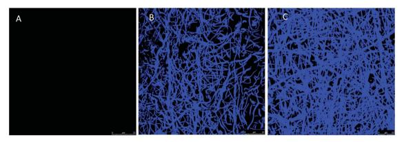
Fig. 3 Confocal laser scanning microscopy images of PAA-PVA fibres (A), nisin-loaded PAA-PVA (N\_3@PAA-PVA, pH 7, (B)) and lysozyme-loaded PAA-PVA (L\_3@PAA-PVA, pH 7, (C)) after conjugation with fluorescamine.
