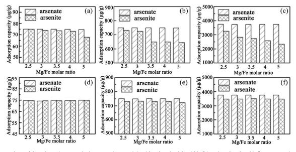
Fig. 8 Comparison of the adsorption capacity between the uncalcined (a-c) and calcined (d-f) iowaites. (a-c) or (d-f) correspond to the initial arsenic concentrations in solution of 150, 1500, and 7500  $\mu$ g L<sup>-1</sup>, respectively (reproduced with permission from ref. 92).
