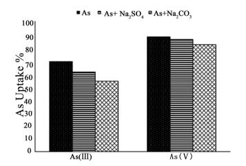
Fig. 10 The effect of competitive anions on the As(III) and As(V) uptakes using the Zn-Al-SO<sub>4</sub> LDH (reproduced with permission from ref. 85).
