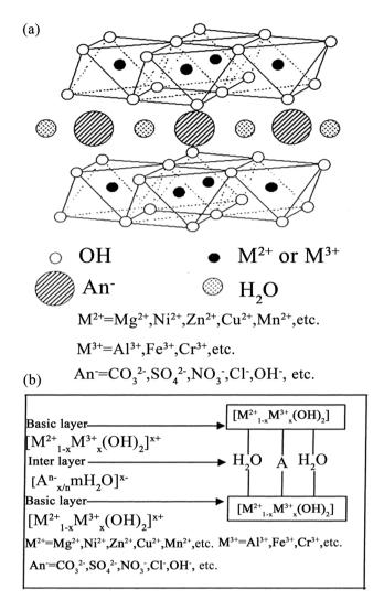
Fig. 1 Structure models for LDHs  $[M_{1-x}^{2+}M_x^{3+}(OH)_2][A^{n-}]_{x/n} \cdot mH_2O$  (a) 3D structure and (b) 2D structure (reproduced with permission from ref. 68)
