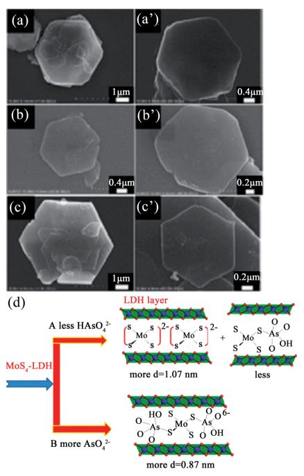
Fig. 6 SEM images of the samples after  $MoS_4$ -LDH adsorption with (a and a') 10 ppm As(|||), (b and b') 300 ppm As(|||) and (c and c') 10 ppm As(v); (d) a scheme showing the dominant phases and possible binding modes of  $MoS_4^{2-}$  with  $HAsO_4^{2-}$  in the LDH gallery (adapted with permission from ref. 89).
