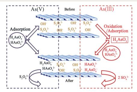
Fig. 5 A schematic diagram of the proposed mechanism for As( $\bowtie$ ) and As( $\bowtie$ ) adsorption on the Mg-Fe-S<sub>2</sub>O<sub>8</sub> LDH (reproduced with permission from ref. 88).
