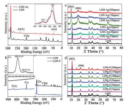
Fig. 4 XPS spectra of the Mg-Al-LDHs before and after the adsorption of (a) As(v) and (b) F<sup>-</sup>; XRD patterns of the Mg-Al-LDHs after the adsorption of (c) As(v) and (d) F<sup>-</sup> with different initial concentrations (adapted with permission from ref. 87).
