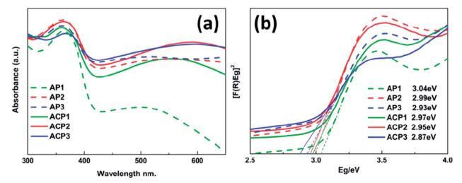
UV-vis diffuse reflectance spectra (a) and Tauc plots with their band gap values (b).
