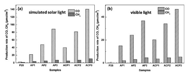
Fig. 7 Evolution of CO and CH<sub>4</sub> yields of different samples under simulated solar light (a) and visible light (b)
