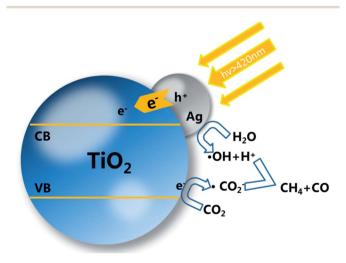
Scheme 2 Schematic of mechanism for photocatalytic process of  ${\rm TiO_2}$  decorated with AgNPs and surface self-doping.
