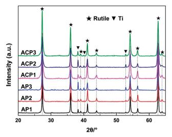
Fig. 1 XRD patterns of the different samples.  $\nabla$ : Ti metal and  $\bigstar$ : rutile phase of TiO<sub>2</sub>.
