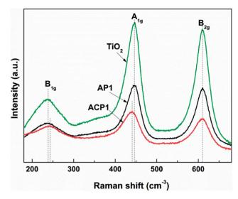
Fig. 6 Raman spectra of the different samples
