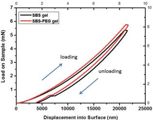
Fig. 7 Nanoindentation load—displacement curves for SBS gel and SBS-PEG gel. Maximum indentation depth applied was 22  $\mu$ m.
