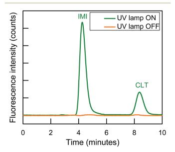
Fig. 3 Isocratic separation of two NNIs and PIF detection at  $\lambda_{ex}/\lambda_{em} =$ 332/368 nm for IMI and  $\lambda_{ex}/\lambda_{em}=353/408$  nm for CLT, respectively.
