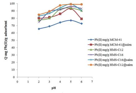
Fig. 9 Influence of pH solution on adsorption of Pb(II) (100 mg L<sup>-1</sup> solutions) onto silicas
