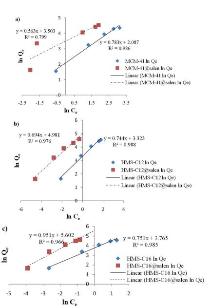
Fig. 12 Freundlich linearized isotherms for Pb(II) sorption onto (a) MCM-41, MCM-41@salen; (b) HMS-C12, HMS-C12@salen, (c) HMS-C16, HMS-C1 C16@salen.
