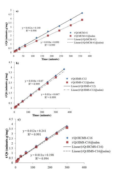
Fig. 14 Pseudo-second order sorption kinetics of Pb(II) onto (a) MCM-41, MCM-41@salen; (b) HMS-C12@salen; (c) HMS-C16 and HMS-C16@salen.
