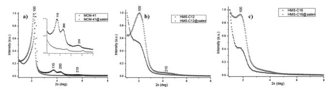
Fig. 6 XRD patterns for the synthesized mesoporous silicas: (a) MCM-41, MCM-41@salen; inset graph: enlargement of the XRD pattern with diffraction planes indices; (b) HMS-C12@salen; (c) HMS-C16@salen.
