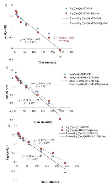
Fig. 13 Pseudo-first order sorption kinetics of Pb(II) onto (a) MCM-41, MCM-41@salen; (b) HMS-C12, HMS-C12@salen; (c) HMS-C16 and HMS-C16@salen
