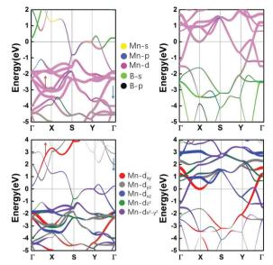
Fig. 3 Atom-projected and orbital-projected band structures of MnB sheets in spin-up and spin-down channels, and the Fermi levels are set to zero
