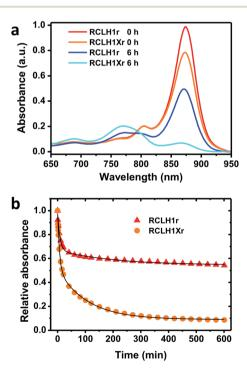
Fig. 6 Thermal stabilities of the RCLH1Xr and RCLH1r proteins. (a) Near-IR absorbance spectra of the pigment-protein solutions before and after heating at 60  $^{\circ}$ C for six hours, (b) decay of the amplitude of the  $Q_y$  absorbance band of the LH1 BChls over a 10 hour incubation at 60  $^{\circ}$ C. The data were fitted with two exponential terms and an offset to illustrate their biphasic nature.
