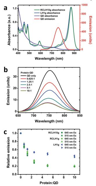
Fig. 4 Quenching of QD emission by the RCLH1Xg or RCLH1g complexes. (a) Absorbance spectra of the RCLH1Xg and LH1g complexes, and absorbance and emission spectra of 6.5 nm-diameter water soluble CdTe QDs, (b) quenching of emission of 50 nM QDs by 31.25–500 nM RCLH1Xg complexes, with excitation at 515 nm, (c) decay of relative QD emission as a function of protein: QD ratio, using data collected at two excitation wavelengths. The data points are means with standard deviation (n = 3).
