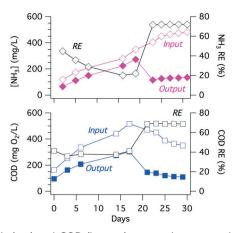
Fig. 7  $\,$  NH $_3$  (top) and COD (bottom) averaged concentrations before (input) and after (output) an electrochemical treatment cycle of 4 hours with respective removal efficiencies (RE) for 30 continuous days of operation of YXG prototype. Day 0 corresponds to the beginning of usage of the prototype.
