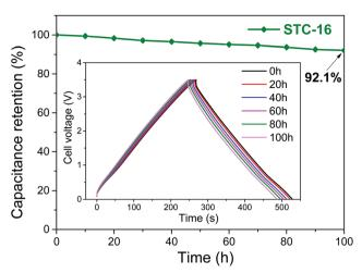
Fig. 4 Floating stability of STC-16 at a specific current of 1 A  $g^{-1}$  for 100 h of floating at 3.5 V. The inset shows the charge/discharge profiles every 20 h. Figures reproduced with permission from ref. 21
