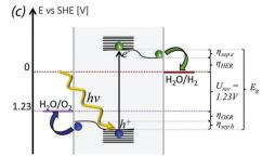
Fig. 1 (a) Toy model of a PV-electrolyser, which after optimization can reach over 15% STH efficiency. (b) Possible geometry of a monolithic PEC-WS device. Elegant, but not good enough. (c) Schematic energetics of PEC-WS
