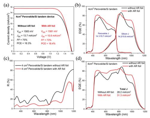
Fig. 6 (a) J-V curves, (b) EQE, (c) reflectance and (d) "total" EQE of the best tandem device (MAPbI<sub>3</sub> = 380 nm) that uses the lightly doped p++ emitter in the Si bottom cell before (black) and after (red) the application of the AR foil. The "total" EQE curve in (d) is the sum of the EQEs from the top perovskite and bottom silicon cells.
