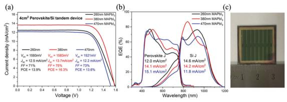
Fig. 2 (a) J-V curves and (b) EQE of the tandem devices with different thicknesses of the MAPbl<sub>3</sub> perovskite layer (260, 380 and 470 nm). (c) A photo of a fabricated 4 cm<sup>2</sup> tandem device.
