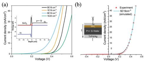
Fig. 3 (a) Simulated dark J-V curves for the  $SnO_2/p++$  silicon interface when the p++ doping concentration is varied. Inset: Corresponding band diagram taking into account the effect of native  $SiO_2$ . (b) Dark J-V characteristics of the Ag/SnO<sub>2</sub>/p++ Si/Ag test device (the inset shows the structure of the test device)
