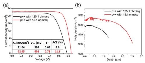
Fig. 4 (a) Current density-voltage (J-V) curves of Si bottom cells that have different p++ emitter profiles (black for 125.1 ohm sq<sup>-1</sup>). (b) Doping profiles of the same cells measured with electrochemical capacitance-voltage measurements.
