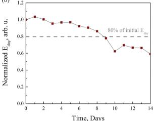
Fig. 1 (a) PCE evolution of the glass/ITO/SnO $_2$ /Cs $_{0.05}$ ((CH $_3$ NH $_3$ ) $_{0.15}$ - $(CH(NH_2)_2)_{0.85})_{0.95}PbI_{2.55}Br_{0.45}/Spiro-OMeTAD/Au$  cell (type I) during two weeks of outdoor exposure to natural sunlight. (b) Evolution of the daily energy output,  $E_{day}$ , generated by this cell, normalized by its value on the first day. For simplicity, we used a constant  $P_{in}$  = 1 Sun for the  $E_{day}$ calculation. All lines are guides for the eye.
