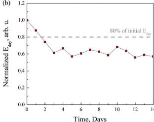
Fig. 2 (a) PCE evolution of type II mini-modules (glass/ITO/TiO<sub>2</sub>/MAPbI<sub>3</sub>/ Spiro-OMeTAD/Au) during their outdoor sunlight exposure. (b) Evolution of the daily energy output generated by this cell. For simplicity, we used a constant  $P_{in} = 1$  Sun for the  $E_{day}$  calculation. All lines are guides for the eye.
