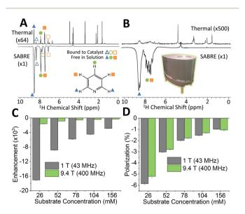
Fig. 2 Comparison of thermally polarized (top) and SABRE hyperpolarized (bottom) <sup>1</sup>H NMR spectra of 52 mM pyridine with 5.2 mM catalyst in methanol- $d_4$  for NMR detection at (A) 9.4 T and (B) 1 T. (C) SABRE enhancement factor,  $\varepsilon$ , and (D) polarization level, P, for the ortho resonance (blue triangle) as a function of substrate concentration with NMR detection at 1 T (gray) and 9.4 T (green). Error bars represent the standard deviation across 5 measurements.
