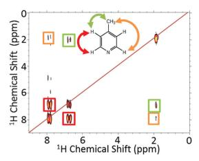
Fig. 6 2D gradient selective COSY coupled with SABRE for 52 mM 4-methylpyridine and 5.2 mM catalyst in methanol- $d_4$ . The COSY measurements used 64 increments over a bandwidth of 500 Hz (11.5 ppm), with single scan transients and re-hyperpolarization between each point. The total experiment time was around 36.4 minutes.
