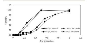
Fig. 4 Validation of the OD sensor – comparison with a Varioskan(R) instrument in 150 and 50 µL of sample dilutions of the green food dye (E143), N = 3
