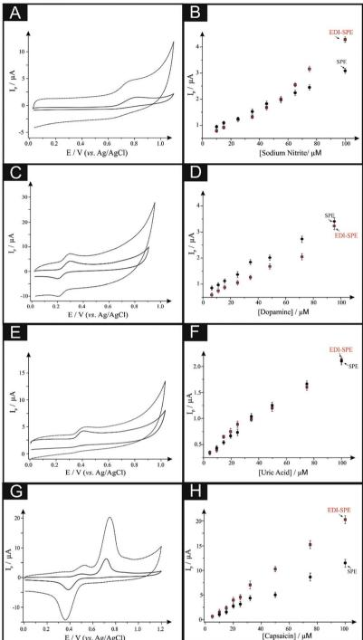
Fig. 2 Cyclic voltammograms utilising EDI-SPEs explored towards the electroanalytical detection of: (A) 50 μM nitrite, (C) 50 μM dopamine, (E) 50 μM uric acid and (G) 50 μM capsaicin obtained for SPEs (solid line) and EDI-SPEs (checked lines). Resulting calibration plots for (B) nitrite, (D) dopamine, (F) uric acid and (H) capsaicin, obtained for SPEs (circles) and EDI-SPEs (squares). In all cases, scan rate:  $0.1 \text{ V s}^{-1}$ .
