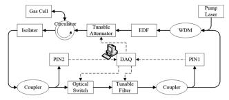
Fig. 4 Schematic of the C<sub>2</sub>H<sub>2</sub> experiment system.
