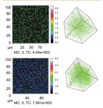
Fig. 1 ToF-SIMS surface imaging of D<sub>2</sub>O at an approximately 150 nm depth in thin films and 3D depth profile plots of glass/CH3NH3Pbl3 films pre-treated with (top) 25% and (bottom) 85% deuterated water in humid environments. MC is the maximum count and TC is the total number of D<sub>2</sub>O counts.
