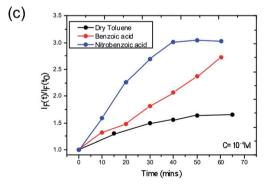
Fig. 3 Superoxide yield plots for  $CH_3NH_3Pbl_3$  where (a) demonstrates the effect on the yield *via* pre-treating the film under no moisture, 25% RH and 85% RH, (b) demonstrates the effect of increasing water content in the toluene solution that houses the superoxide reactive probe and (c) shows the impact of acid strength on the superoxide yield, where benzoic acid and nitrobenzoic acid are doped into the toluene solution.
