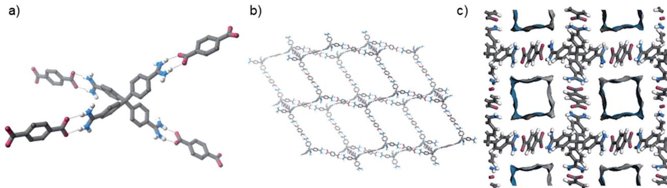
Fig. 2 Views of the solid state structure of  $[2 \cdot (\text{TP})_2]_n$ : (a) view showing hydrogen bonding interactions, (b) view of one of the interpenetrating nets, (c) view down the  $c$ -axis highlighting  $\text{N}_2$ -accessible pores (solvent molecules and some hydrogen atoms are omitted for clarity, see Fig. S23† for additional views of the structure).
