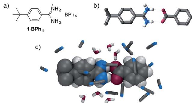
Fig. 1 (a) Structure of model compound  $1 \cdot \text{BPh}_4$ , (b) X-ray crystal structure of  $1 \cdot \text{benzoate}$ , (c) representative snapshot from MD simulations of binding of  $1^+$  and benzoate in 20 mM 95 : 5  $\text{CH}_3\text{CN} : \text{H}_2\text{O}$ .
