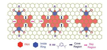
Scheme 1 Molecular structure of the twisted derivatives 1c and 2d along with the planar derivative 3c (arrows indicate the cove and bay regions in the derivatives).
