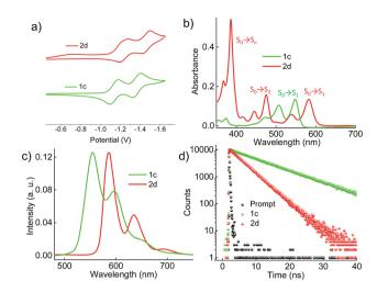
Fig. 3 (a) Electrochemical measurement of the derivatives in dry DCM with reference to the Fc/Fc<sup>+</sup> electrode, (b) UV-Vis absorption spectra, (c) emission ( $\lambda_{ex}=480$  nm), and (d) time-dependent fluorescence spectra ( $\lambda_{ex}=480$  nm and monitored at the respective emission maxima) of the derivatives 1c and 2d in toluene.
