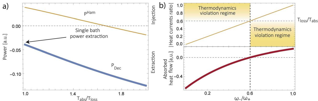
Fig. 4 (a) Predicted power extraction for the decay ( $P^{\text{Dec}}$ , thick blue line) and the Hamiltonian ( $P^{\text{Ham}}$ , thin yellow line) transfer schemes. (b) Absolute value of the heat currents ratio (yellow thin line) for the Hamiltonian transfer scheme (top) and  $J_{\text{abs}}^{\text{Ham}}$ , (bottom, thick red line).
