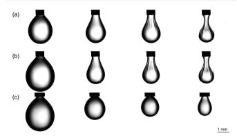
Fig. 8 Transmission optical micrographs of the pendant droplet during IFT measurements of continuous aqueous  $A_2-B_3-CB[8],$  and droplet of 0.001 wt% K $^-$  in FC-40. From left to right, (a) equilibrated 5  $\mu L$  droplet pumped in and exhibiting a buckled phase change; (b) droplet after subsequent pumping out to 8.5  $\mu L$  followed by immediate pumping in; (c) droplet containing 0.01 wt% K $^+$  in FC-40 and subsequent pumping in.
