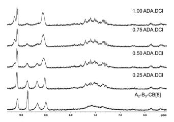
Fig. 4  $^{1}$ H NMR spectra in D<sub>2</sub>O of A<sub>2</sub>-B<sub>3</sub>-CB[8] hyperbranched supramolecular polymer upon titration with up to 1 molar equivalent of ADA · DCI relative to CB[8].
