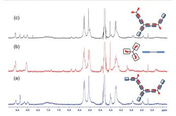
Fig. 3  $^{1}$ H NMR spectra in D<sub>2</sub>O of (a) A<sub>2</sub>-B<sub>3</sub>-CB[8] hyperbranched supramolecular polymer in its equilibrium state; (b) after 1 h of UVA exposure; (c) after subsequent heating at 80 °C for 6 h. Note, upon heating the azobenzene is >99% E isomer, higher than that originally present in (a).
