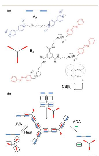
Fig. 1 (a) Chemical structures and schematic representations of CB[8], and the ditopic ( $A_2$ ) and tritopic ( $B_3$ ) monomers used in this work. (b) Overview of the proposed assembly process;  $A_2$  is first complexed with CB[8] (2 eq.), and then mixed with  $B_3$  (0.67 eq.) to form the SHP. This SHP can be disassembled in response to either (i) reversible photoisomerisation of the azobenzene (left), or (ii) introduction of a competitive guest (right).
