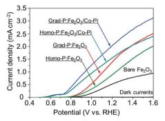
Fig. 4 I-V characteristics of bare Fe<sub>2</sub>O<sub>3</sub>, homo-P:Fe<sub>2</sub>O<sub>3</sub>, grad-P:Fe<sub>2</sub>O<sub>3</sub>, homo-P:Fe<sub>2</sub>O<sub>3</sub>/Co-Pi and grad-P:Fe<sub>2</sub>O<sub>3</sub>/Co-Pi photoanodes measured in 1 M KOH solution under AM 1.5G illumination (100 mW cm<sup>-2</sup>). The dark currents are negligible for all samples.
