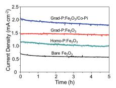
Fig. 10 Stability test of bare  $Fe_2O_3$ , homo-P: $Fe_2O_3$ , grad-P: $Fe_2O_3$  and grad-P: $Fe_2O_3/Co$ -Pi photoanodes for 5 h at 1.23 V (vs. RHE) under AM 1.5G illumination.
