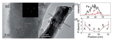
Fig. 2 (a) HRTEM image of a selected area of grad-P: $Fe_2O_3$ ; inset of (a) is the SAED pattern; (b) TEM image of a single grad-P: $Fe_2O_3$  bundle; (c) the P element distribution in a  $Fe_2O_3$  nanobundle (line in image b); (d) the P element concentration along the radial direction (dots in image b) (the error bar represents the standard deviation).
