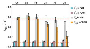
Fig. 4 Excess charge ( $\delta^-$ ) or lack of charge ( $\delta^+$ ) on H, O, and O–O in \*OH and \*OOH. While the charges of H in \*OH (light blue), H in \*OOH (brown), and O in \*OH (gray) are relatively constant for the different metal centers, that of O-O in \*OOH (orange) undergoes large changes as the metal ion goes from Cr to Cu. The red dashed lines correspond to the average values of O and H in \*OH. Error bars are provided to show the effect of the ring ligands.
