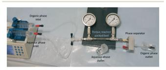
Fig. 4 Photograph of the experimental setup for chemical mass transfer measurements.
