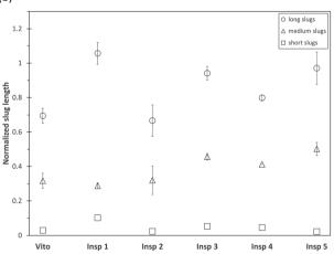
Fig. 7 Normalized averaged slug lengths of the continuous water phase (a) and dispersed toluene phase (b) for a total flow rate of 3 ml min<sup>-1</sup>. The bars indicate the standard deviation in the measured slug lengths.
