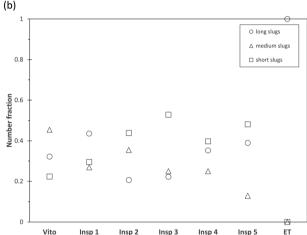
Fig. 8 Distribution of slug sizes of the continuous water phase (a) and dispersed toluene phase (b) for a total flow rate of 3 ml min<sup>-1</sup>.
