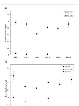
Fig. 5 Normalized averaged slug lengths of the continuous water phase (a) and dispersed toluene phase (b) for a total flow rate of 1 ml min<sup>-1</sup>. The bars indicate the standard deviation in the measured slug lengths.
