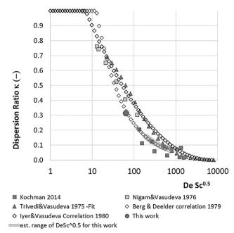
Fig. 4 The dispersion ratio  $\kappa$  vs. DeSc<sup>0.5</sup> for various literature data. Where possible data have or correlations have been taken from the papers. If the data could not be retrieved and no correlation was given the data has been fitted with a line that visually represents the data well.
