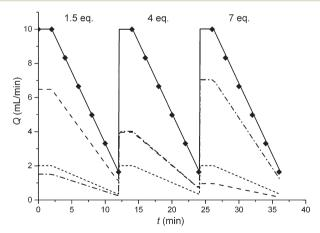
Fig. 2 Changes in volumetric flow rate over time, where  $Q_{\rm P1}$ ,  $Q_{\rm P2}$ ,  $Q_{\rm P3}$  and  $Q_{\rm total}$  were for ..... pump 1 (Ar in EtOH), --- pump 2 (EtOH), --- pump 3 (pyrrolidine in EtOH), --- total volumetric flow rate, and  $\Phi$  HPLC injection respectively. The linear flow ramps correspond to pyrrolidine 2 to 2,4-difluoronitrobenzene 1 molar ratios: (i) 1.5:1, (ii) 4:1 and (iii) 7:1 using  $Q_{\rm total}$  from 10 to 1.5 mL min $^{-1}$ .
