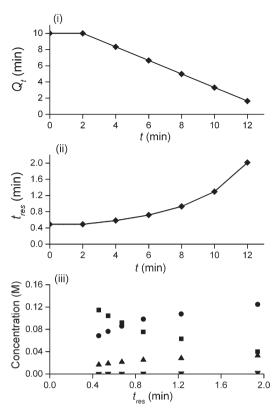
Fig. 3 i) Total volumetric flow rate  $(Q_{total})$  change throughout the duration of a ramp,  $\bullet$  HPLC injection; (ii) residence time,  $\tau$ , as a function of operation time, t; (iii) resulting concentration-residence time profile generated from a typical multi-step reaction scenario, 2,4-DF 1, • ortho-3, • para-4, ▼ bis-5
