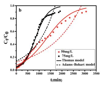
Fig. 7 Experimental and predicted breakthrough curves of  $Cr(v_1)$  removal by CPA-2 using fixed-bed (a) different flow rates ( $C_0 = 50 \text{ mg L}^{-1}$ , H = 8 cm, pH = 2, T = 298 K); (b) different initial  $Cr(v_1)$  concentrations ( $Q = 1 \text{ mL min}^{-1}$ , H = 8 cm, pH = 2, T = 298 K).
