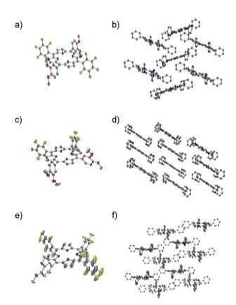
Fig. 1 ORTEP molecular diagrams of (a) P1, (c) P2 and (e) P3 where the solvent molecules and hydrogens have been omitted for clarity. Thermal ellipsoids are also shown at 50% probability for P1 and P2 and 35% probability for P3. Crystal packing diagrams for (b) P1, (d) P2 and (f) P3 where the solvent molecules and hydrogen, oxygen and fluorine atoms have been omitted for clarity. Thermal ellipsoids are also shown at 50% probability for P1 and P2 and 35% probability for P3.
