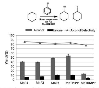
Fig. 5 Cyclohexane oxidation reaction using PhIO catalysed by MnP1, MnP2, MnP3, MnTPFPP and MnTDMPP. Catalyst/PhIO/Substrate molar ratio =1:10:1000. The product yields for cyclohexanol (alcohol) and cyclohexanone (ketone) were calculated based on the amount of PhIO used in the reactions. Results represent reactions performed in duplicate.
