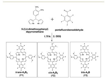
Scheme 1 Schematic representation of the free-base porphyrins preparation.
