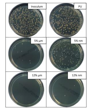
Fig. 8 Images of agar plates showing the results of antibacterial tests against Staphylococcus gallinarum (contact time 24 hours).
