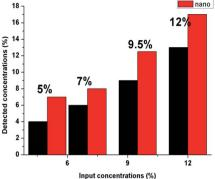
Fig. 6 Difference between input and detected concentrations of micro- and nanoparticles of CuO.
