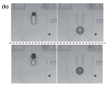
Fig. 9 Droplet coalescence systems to obtain molecular gradients. (a) Simultaneously generation of individual droplets controlled by external electrovalves (reproduced from ref. 172 with permission from the Royal Society of Chemistry). (b) Pillars used to realize fusion without the demand for the synchronization, while the upper line and lower line show passive coalescence with different volume ratios, respectively (reproduced from ref. 174 with permission from Springer).
