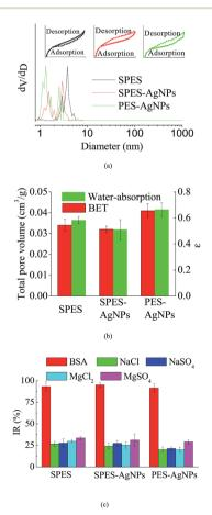
Fig. 4 (a) BET results; (b) porosity properties; and (c) interception capacity of the prepared membranes.
