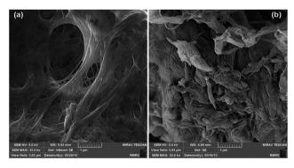
Fig. 5 FE-SEM picture of neat NFC (a) and NFC 4.0 TMSQI (b).
