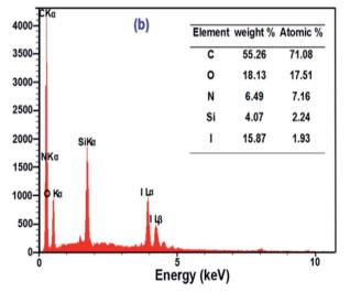
Fig. 4  $\,$  EDX spectra and tabulated results of neat NFC (a) and NFC 4.0 TMSQI (b).
