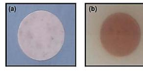
Fig. 8 Zone of inhibition test for neat NFC (a) and NFC 4.0 TMSQI (b) against S. aureus.
