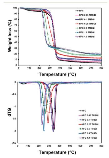
Fig. 7 TGA (a) and DTG (b) of neat NFC and NFC grafted with 0.05-4 g TMSQI.
