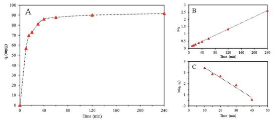
Fig. 7 Effect of time on the adsorption capacity (A), the fitting results of the experimental adsorption kinetic data in terms of pseudo-first-order (B) and pseudo-second-order (C) models (pH: 3,  $Cr(v_1)$  concentration: 100 mg  $g^{-1}$ , volume of  $Cr(v_1)$  solution: 40 mL, adsorbent dose 0.5 g  $L^{-1}$ , and temperature: 298 K)
