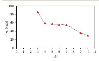
Fig. 6 Influence of initial pH of solution on the adsorption capacity of Cr(vı). Mass of SMGO hybrids = 0.5 g L $^{-1}$ , initial concentration of Cr(vı) = 100 mg L $^{-1}$ , contact time = 60 min, volume of Cr(vı) solution = 40 mL, temperature = 20 °C.
