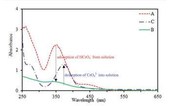
Fig. 9 UV-Vis absorption spectra of the (A) initial solution of Cr(vi) (200 mg  $L^{-1}$ ) at pH = 3, (B) adsorption process at T=318 K, and contact time = 60 min (C) desorption process at pH = 10, T = 298 K, and contact time = 60 min.
