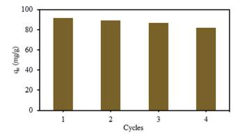
Fig. 12 Recycling of SMGO for the adsorption of Cr(vi). The concentration of SMGO was 1.0 mg  $L^{-1}$ , initial concentration of  $Cr(v_1) =$ 100 mg  $L^{-1}$ , temperature = 298 K, contact time = 60 min, pH = 3.
