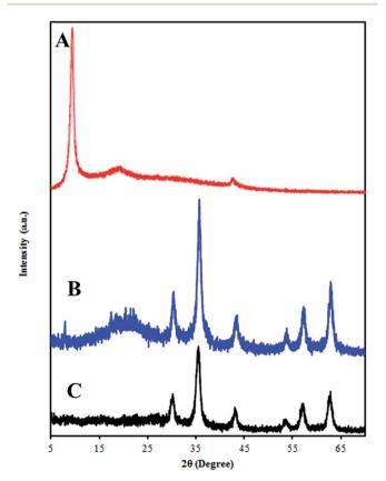
Fig. 2 XRD patterns of GO (A), SMGO (B) and (C)  $Fe_3O_4$ . The patterns of SMGO hybrids show diffraction peaks indexed to (220), (311), (400), (422), (511), and (440) planes appearing at  $2\theta=30.40^\circ$ ,  $35.67^\circ$ ,  $43.33^\circ$ ,  $53.24^\circ$ ,  $57.34^\circ$ , and  $62.85^\circ$ , respectively. These matched the characteristic peaks for  $Fe_3O_4$  in the standard PDF card in the X-ray diffraction atlas (JCPDS card 19-0629) issued by the International Powder Union.
