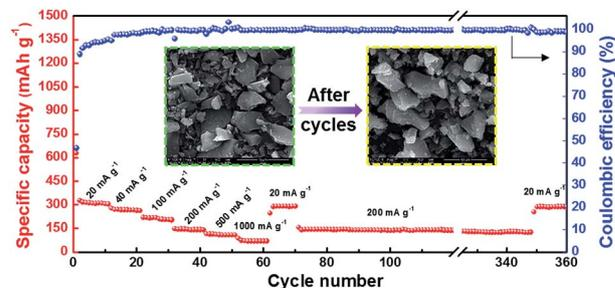
**Fig. 8** Discharge capacities of HC-1000 at different current densities of 20, 40, 100, 200, 500 and 1000  $mA g^{-1}$ , respectively. A long-term cycling performance is recorded from the 70<sup>th</sup> to the 350<sup>th</sup> cycles at 200  $mA g^{-1}$  and SEM images of the HC-1000 electrodes before and after 360 cycles.
