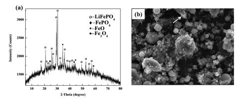
Fig. 5 XRD patterns and SEM image of spent LiFePO<sub>4</sub> after separation: (a) many impurity phases including FePO<sub>4</sub>, FeO and Fe<sub>3</sub>O<sub>4</sub>; (b) irregular particle with many agglomerations.
