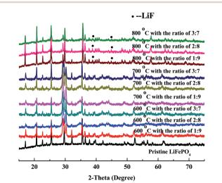
Fig. 7 XRD patterns of regenerated materials with doping new LiFePO\_4 at different temperature and ratio.
