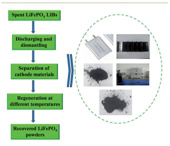
Fig. 1 The flowchart of regeneration process for spent LiFePO $_4$  LIBs in this work.
