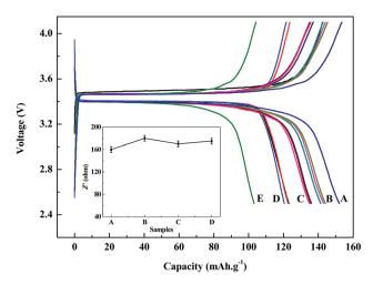
**Fig. 9** Discharge/charge voltage and impedance profiles of regenerated LiFePO<sub>4</sub> at a current density of 0.1C: (A) commercial LiFePO<sub>4</sub>; (B) 700 °C with the ratio of 1 : 9, 2 : 8, 3 : 7; (C) 600 °C with the ratio of 1 : 9, 2 : 8, 3 : 7; (D) 800 °C with the ratio of 1 : 9, 2 : 8, 3 : 7; (E) regenerated without doping new LiFePO<sub>4</sub>.
