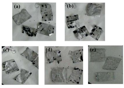
Fig. 3 The dissolution phenomena of cathode plates in different solvents: (a) DMSO; (b) acetone; (c) DMF; (d) NMP; (e) DMAC.
