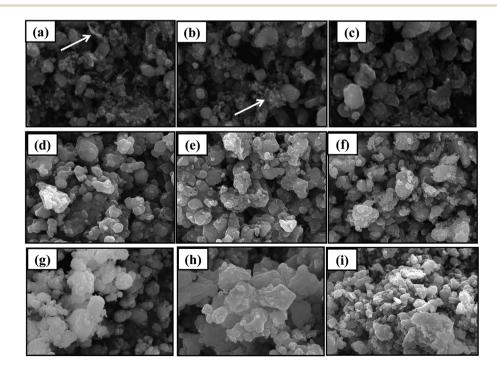
Fig. 8 SEM images of regenerated materials with doping new LiFePO<sub>4</sub> at different temperature and ratio: (a-c) 600 °C with doping at 1 : 9 to 3 : 7; (d-f) 700 °C with doping at 1 : 9 to 3 : 7; (d-f) 700 °C with doping at 1 : 9 to 3 : 7.
