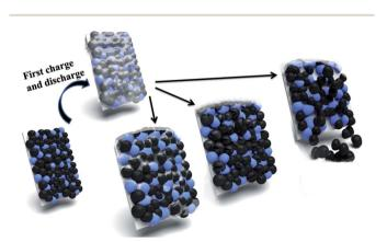
Fig. 6 Illustration of failure mechanism of LiFePO<sub>4</sub> for Li-ion batteries: breakdown of SEI film; decomposition of LiFePO<sub>4</sub>; falling of cathode materials.
