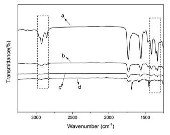
Fig. 4 ATR-FTIR spectra of the film-VH (a) contained 50% ADIm, (b) contained 25% ADIm, (c) contained 10% ADIm, and (d) contained 0% ADIm.
