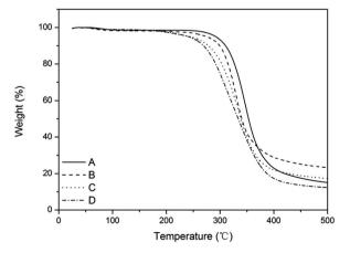
Fig. 6 TGA curve of films with variable content of alkyl chain. (A) Content of ADIm is 0, (B) content of ADIm is 10%, (C) content of ADIm is 25%, and (D) content of ADIm is 50%.
