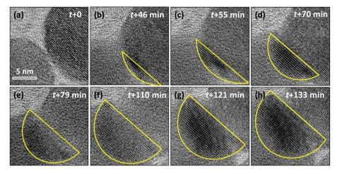
Fig. 4 (a-h) Time dependence of the in situ epitaxial growth of GdF<sub>3</sub> on NaGdF<sub>4</sub> at the interface induced by a focused electron beam with a current density of 40 pA cm $^{-2}$ . The scale bar in all figures is 5 nm. GdF<sub>3</sub> layers are marked with yellow lines for a guide to the eye.
