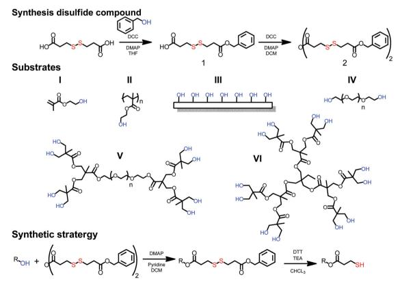
Fig. 1 Synthesis of unsymmetrical disulfide, selected substrates: I HEMA monomer, II pendant group polymer Poly HEMA, III surface (filter paper), VI linear telechelic PEG, V 2,2-bismethylol propionic acid (bis-MPA) based linear dendritic hybrids, VI bis-MPA-based dendrimers and general esterification and deprotection strategy used to convert hydroxide functional substrates to thiol functionality.
