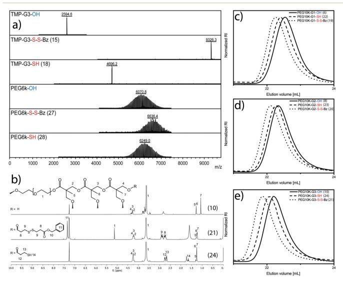
Fig. 2 Selection of analytical data from various substrates. (a) MALDI-TOF-MS of TMP-G3-OH, TMP-G3-S-S-Bz, TMP-G3-SH, PEG6k-OH, PEG6k-S-Bz and PEG6k-SH. (b) <sup>1</sup>H-NMR data for PEG10k-G3-OH, PEG10k-G3-S-Bz and PEG10k-G3-SH. SEC data collected in DMF for: (c) PEG10k-G1-OH, PEG10k-G1-S-Bz and PEG10k-G3-SH. (e) PEG10k-G3-OH, PEG10k-G3-S-Bz and PEG10k-G3-SH. (e) PEG10k-G3-OH, PEG10k-G3-S-S-Bz and PEG10k-G3-SH.
