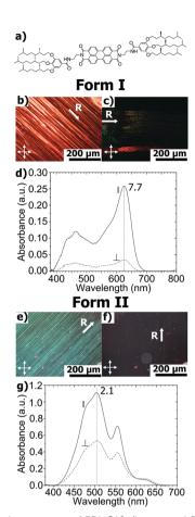
Fig. 1 (a) Molecular structure of PBI-C10. (b, c, e and f) Polarized optical microscopy using crossed polarizers and polarized UV-vis spectroscopy (d and g) of highly oriented PBI-C10 films of J-type aggregate i.e. form I (b-d) and H-type aggregates of form II (e-g). The UV-vis spectra were recorded for parallel ( $\parallel$ ) and perpendicular ( $\perp$ ) orientation of the incident polarized light with respect to the rubbing direction.
