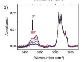
**Fig. 3** Polarized infrared spectra of oriented PBI-C10 thin films of form I in the regions of the amide 1 (a) and of the amide A (b). Polarization varies by 15° steps (from 0° (black) to 90° (red)). 0° (90°) corresponds to the electric field E parallel (perpendicular) to the rubbing direction R, respectively. The inset shows the microscopy image of the investigated area whereas the white arrow highlights the rubbing direction (R).
