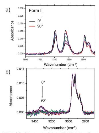
**Fig. 5** Polarized infrared spectra of oriented PBI-C10 thin films of form II. Polarization varies by 15° steps (from  $0^{\circ}$  (black) to  $90^{\circ}$  (red)).  $0^{\circ}$  corresponds to the electric field *E* parallel to the fiber direction (rubbing direction).
