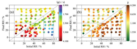
Fig. 3 (a) Exponential folding time, τ, of particle radius responses of ternary sucrose/glucose particles (1:1 mass ratio) to 172 step changes in RH, mapped over initial and final values. (b) The stretched exponential parameter,  $\beta$ , extracted for the same transitions by allowing it to vary during the fitting process.
