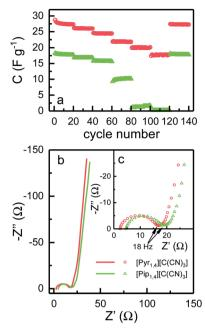
Fig. 6 (a) Specific capacitance obtained from galvanostatic chargedischarge cycling at the different rates 0.5, 1.0, 2.0, 5.0, 7.5, 10 and back to 0.5 A g<sup>-1</sup>. (b) Nyquist plots from EIS measurements and (c) inset showing high frequency semi-circle.
