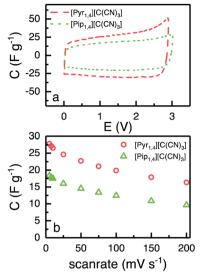
Fig. 5 (a) CVs of EDLC containing [Pyr<sub>1.4</sub>][C(CN)<sub>3</sub>] (red) and [Pip<sub>1.4</sub>][C(CN)<sub>3</sub>] (green) at 5 mV s<sup>-1</sup>, form 0 to 2.9 and 3.0 V, respectively. (b) Calculated capacitance from CVs at different scanrates.
