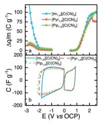
**Fig. 4** Electrochemical stability window determination. (a) difference between  $q_{\rm charge}$  and  $q_{\rm discharge}$ . (b) CV at determined limit voltage for positive and negative sweep for the ILs  $[{\rm Im}_{1,4}][{\rm C(CN)_3}]$  (blue),  $[{\rm Pyr}_{1,4}][{\rm C(CN)_3}]$  (red) and  $[{\rm Pip}_{1,4}][{\rm C(CN)_3}]$  (green).
