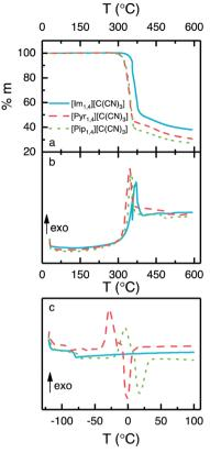
Fig. 2 Thermal analyses of ILs containing [C(CN)<sub>3</sub>] anion, (a) TGA, (b) DSC measured during TGA and (c) DSC.
