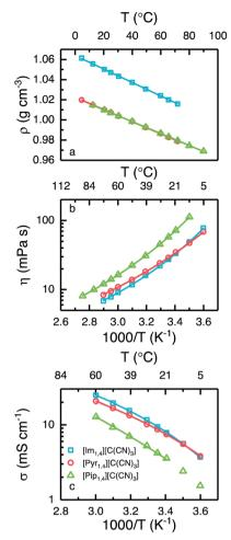
Fig. 3 (a) Density, (b) viscosity and (c) ionic conductivity of the ionic liquids  $[Im_{1,4}][C(CN)_3]$  (blue),  $[Pyr_{1,4}][C(CN)_3]$  (red) and  $[Pip_{1,4}][C(CN)_3]$  (green). Lines in (a) represent density linear fits, and (b) and (c) represent the best VTF fits.
