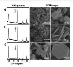
Fig. 11 PXD patterns and SEM images for nano-MH synthesised from: (a) MgCl<sub>2</sub> (b) MgSO<sub>4</sub> and (c) MgO precursors respectively. Reprinted with permission from X. Pan, Y. Wang, Z. Chen, D. Pan, Y. Cheng, Z. Liu, Z. Lin and X. Guan, ACS Applied Materials and Interfaces, 2013, 5, 1137–1142. Copyright 2013 American Chemical Society.<sup>16</sup>
