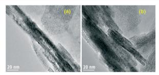
Fig. 3 TEM images of (a) unmodified and (b) poly(ethylene-co-acrylic acid)-modified  $Mg(OH)_2$  nanorods grown by continuous flow hydrothermal processing. Reprinted from *Powder Technology*, **278**, S. Elbasuney and S. F. Mostafa, Continuous flow formulation and functionalization of magnesium di-hydroxide nanorods as a clean nano-fire extinguisher, 72–83, copyright 2015, with permission of
