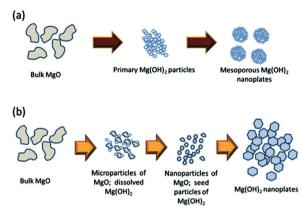
Fig. 9 Proposed growth processes for (a) conventional hydrothermal synthesis proposed by Yu et al. 11 and (b) MW-hydrothermal synthesis proposed by Hanlon et al.<sup>6</sup> reproduced from ref. 6 with permission from the Royal Society of Chemistry.
