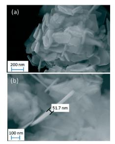
Fig. 8 (a) SEM micrograph of hexagonal nanoplates of Mg(OH)<sub>2</sub> obtained in 4 minutes at 800 W; (b) SEM micrograph showing the thickness of individual nanoplates from the same sample. Reproduced from ref. 6 with permission from the Royal Society of Chemistry.
