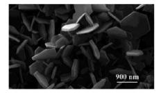
Fig. 2 High magnification SEM images of hexagonal mesoporous Mg(OH)<sub>2</sub> nanoplates obtained *via* surfactant-free hydrothermal synthesis. Reprinted with permission from J. C. Yu, A. Xu, L. Zhang, R. Song and L. Wu, *J. Phys. Chem. B*, 2004, **108**, 64–70. Copyright 2004 American Chemical Society.<sup>11</sup>
