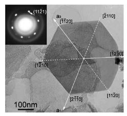
Fig. 4 TEM image and selected area electron diffraction (SAED) pattern (inset) of a regular hexagonal Mg(OH)2 nanoflake synthesised from Mg(NO<sub>3</sub>)<sub>2</sub> and N<sub>2</sub>H<sub>4</sub>·H<sub>2</sub>O. Reprinted from Materials Chemistry and Physics, 112, D. Jin, X. Gu, X. Yu, G. Ding, H. Zhu and K. Yao, Hydrothermal synthesis and characterization of hexagonal Mg(OH)<sub>2</sub> nano-flake as a flame retardant, 962-965, copyright 2008, with permission of Elsevier.31
