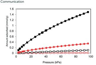
Fig. 3  $CO_2$  and  $N_2$  adsorption isotherms for 1 and 2 at 0 °C (black squares,  $CO_2$  for 1; open squares,  $N_2$  for 1; red circles,  $CO_2$  for 2; open circles,  $N_2$  for 2).
