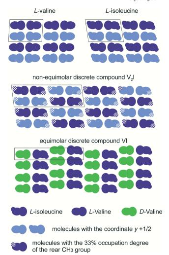
Fig. 10 Schematic representations of molecular packing in crystal structures of Val, Ile, and non-equimolar compound  $V_2I$  in the L-Val-L-Ile system and the equimolar compound VI in the D-Val-L-Ile system.
