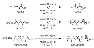
**Scheme 1** Chemoenzymatic polymerization of Aib-containing monomers using papain.
